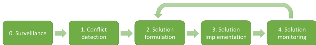
Figure 5. Separation provision process flowchart (from [32]).
